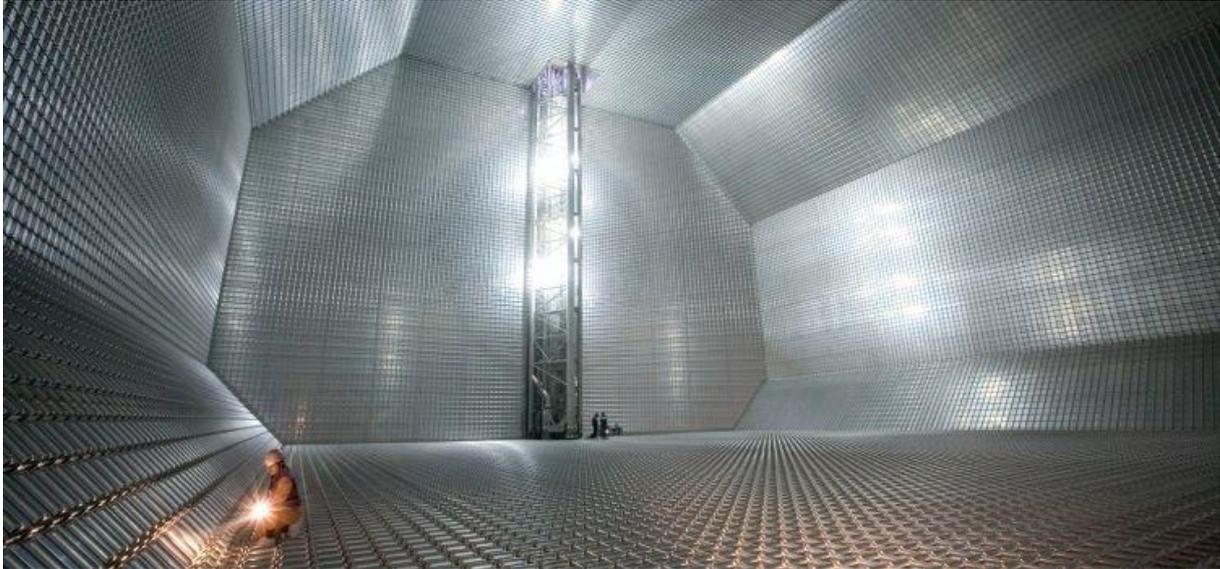
An LNG carrier tank equipped with GTT technology. PERFECt partner GTT wants to break into container shipping (credit: Samsung Heavy Industries)
